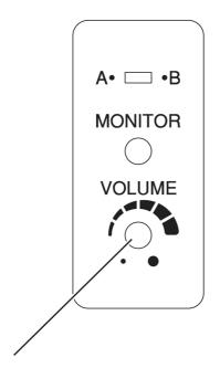
There is no dedicated ON/OFF switch. Use the volume control to turn ON/OFF the melodies. To silence the melodies completely, adjust the volume control knob to the leftmost position.
